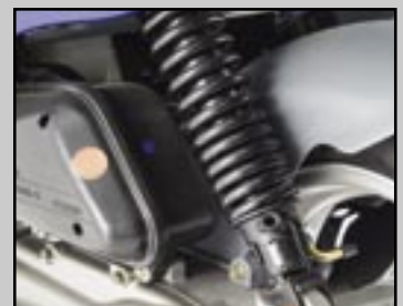
Double spring rear suspension
